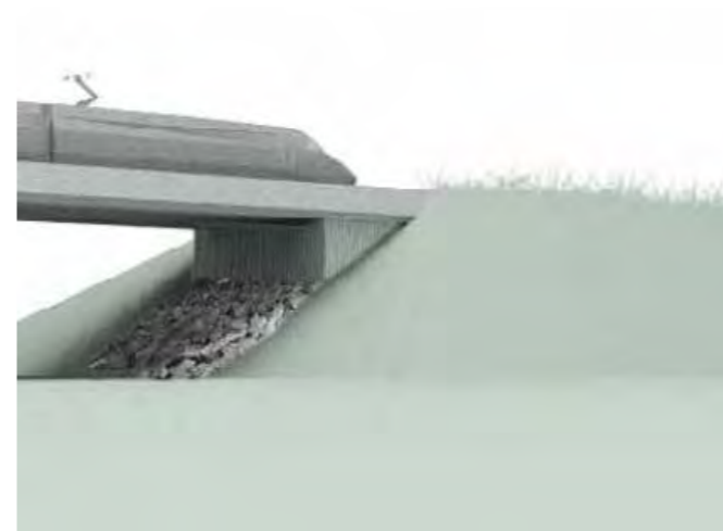
Sloped abutments with tapered textured materials blend into landscape and soft treatment to top of embankments blend well into skyline ©CRT
