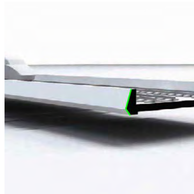
Chamfered edge to deck creates slender appearance ©CRT
